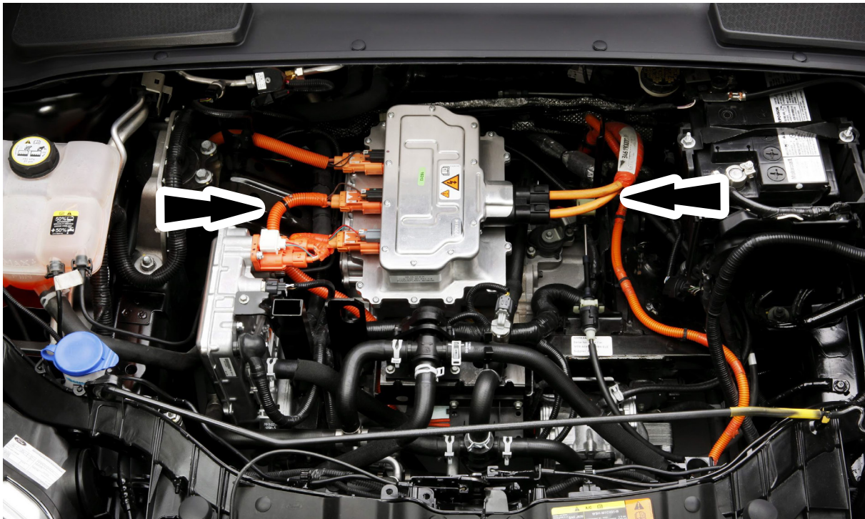
Orange high-voltage cabling from the high-voltage battery packs.
